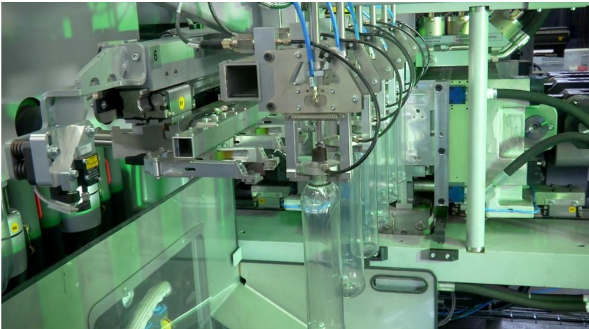
The still-hot preforms are blown into bottles, which go into the cooling tunnel in the next production step. At the end of the processing chain, the recyclate PET bottle is used domestically and internationally.
